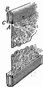
Fig. 184—Section Showing Metal Frame Cheese-Cloth and Clamping Frame
