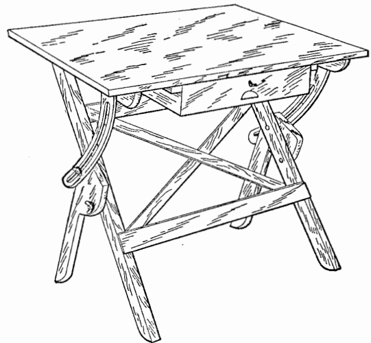
Fig. 3.—Adjustable Drafting Table for Shop Use
